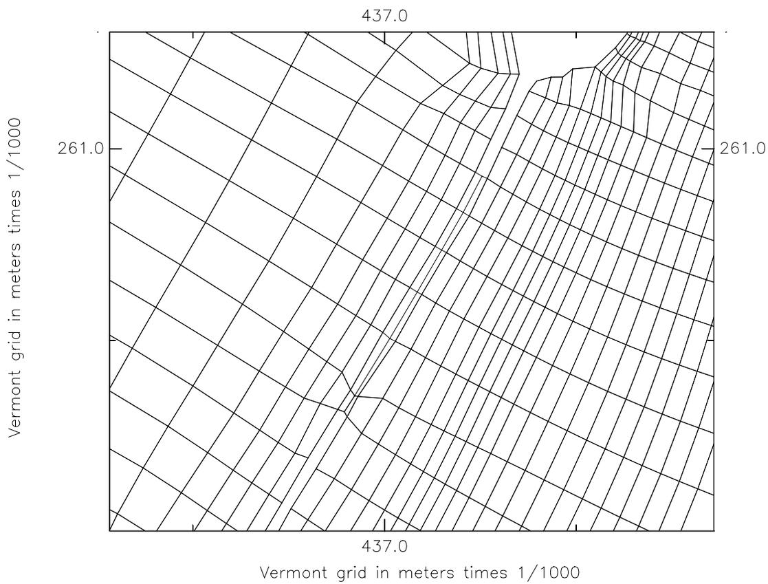
Upper grid shows the details in Carry Bay and near the shore where the grids are smaller. The lower grid is near the north section of the causeway showing the section removed in the simulation of "no-north"
