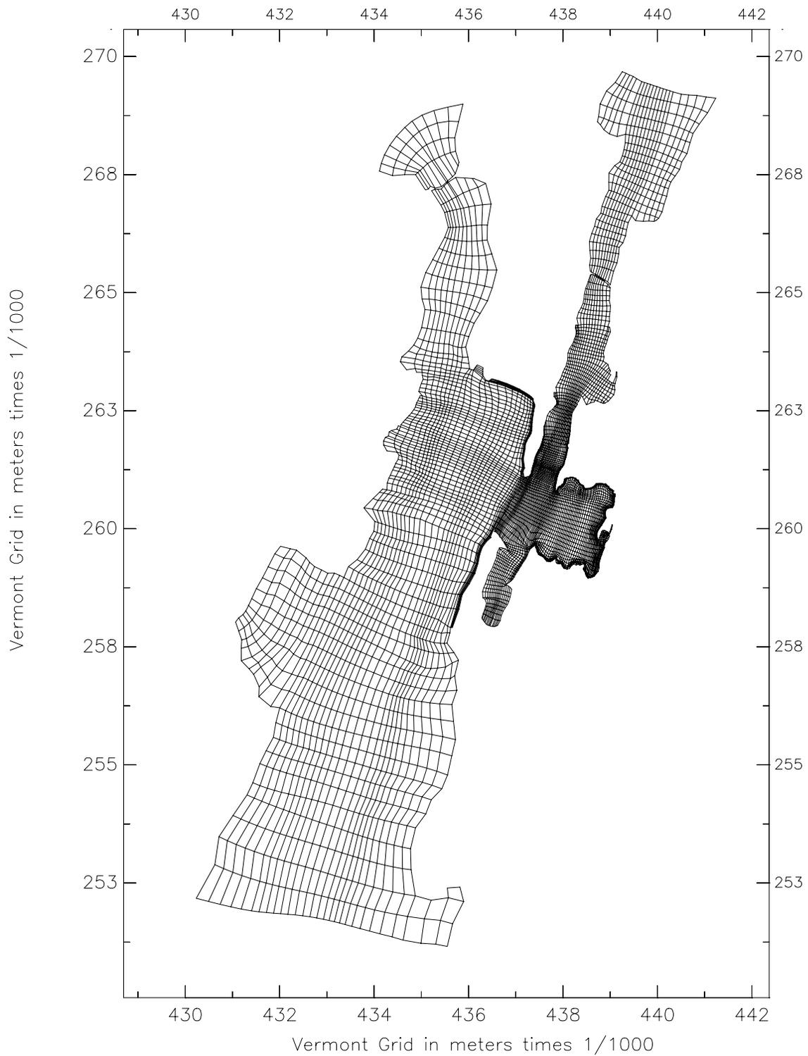
This is the entire computational grid. Near Carry Bay the grid cell size decreases to obtain better resolution. There are about 8860 individual cells in the grid.
