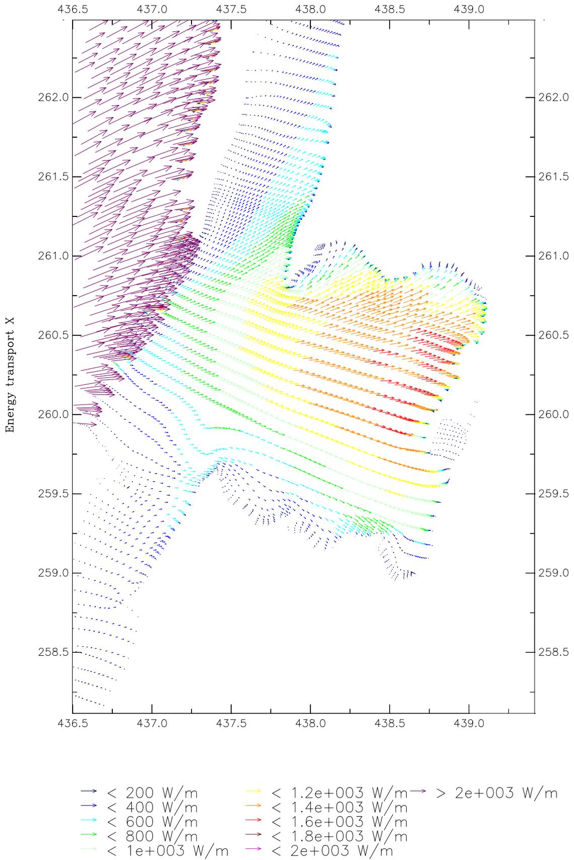
Energy transport vectors for 70 mph west wind with causeway in-place. Compare with Figure 36 – north section removed.
