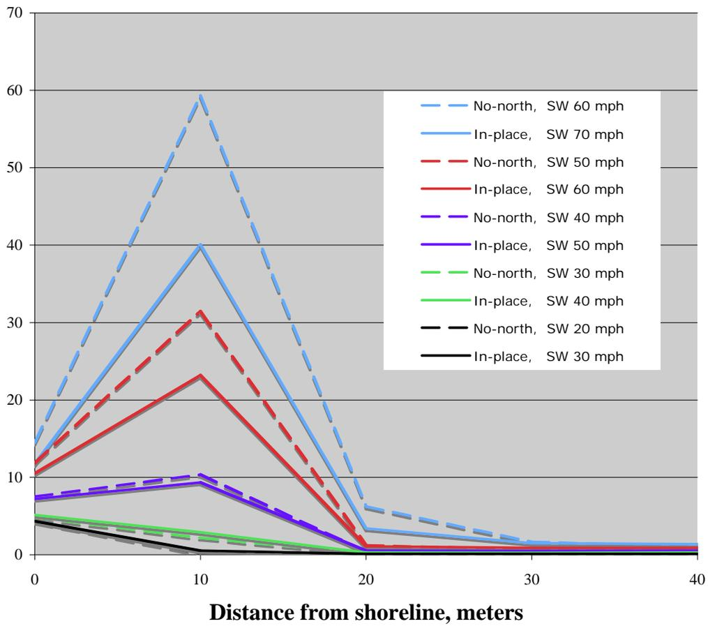
Figure 5.2 Energy dissipation versus distance from the shoreline, north of Blockhouse Point.
