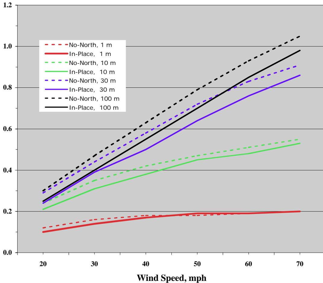
**Figure 5.3 Predicted significant wave heights versus wind speed, east shore of Carry Bay.**
