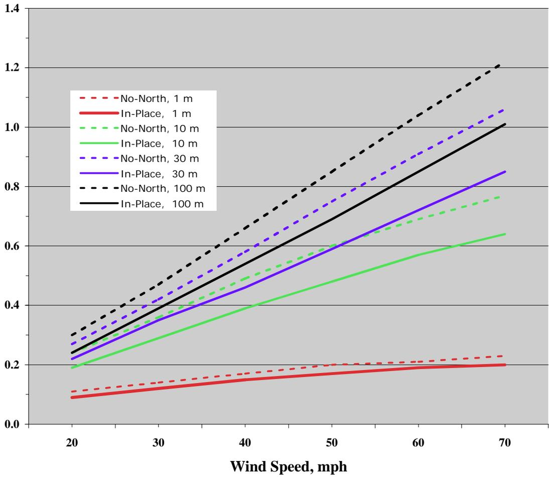
**Figure 5.1 Predicted significant wave heights versus wind speed north of Blockhouse Point.**
