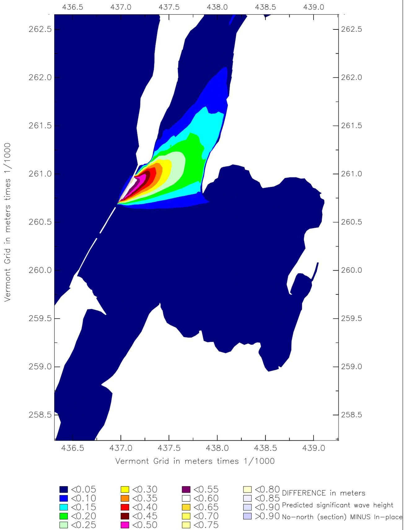
Colors represent DIFFERENCE in predicted significant wave heights in meters between no-north section and in-place causeway predictions.
