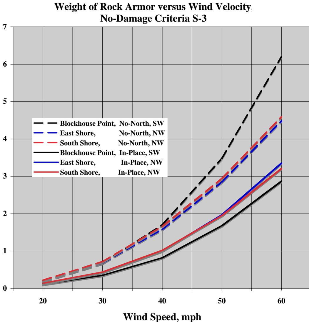
**Figure 5.4** Calculated weight of rock armor versus wind speed, Carry Bay beaches.
