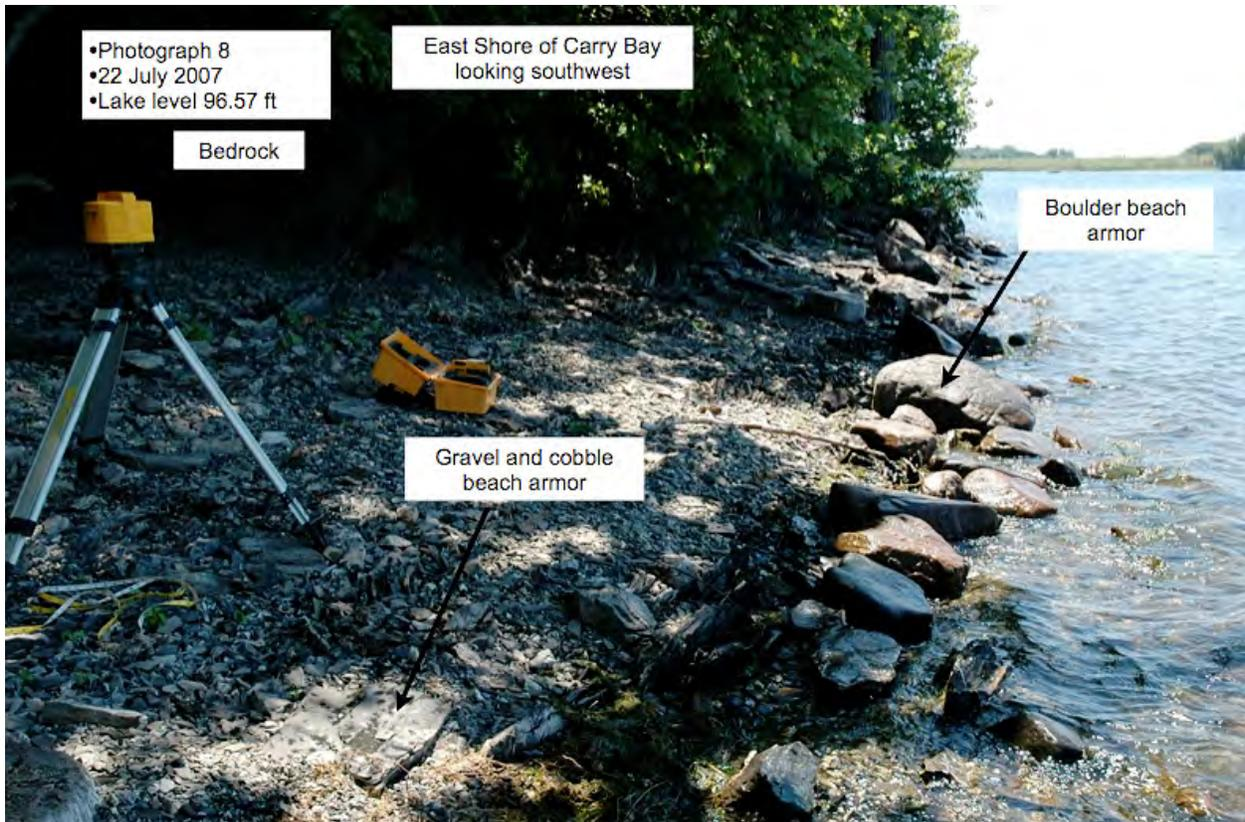
**Photograph 8** - This picture was taken during the survey of beach slopes on July 22, 2007. The instrument on the tripod is a laser level. The beach is armored with boulders with cobbles.
