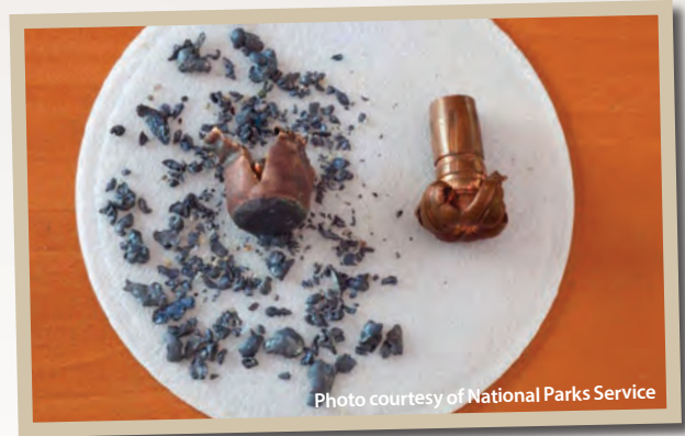
A recovered .270 caliber copper jacket lead-core bullet (left) is heavily fragmented compared to the solid copper bullet (right) that retained its original shape upon impact.
