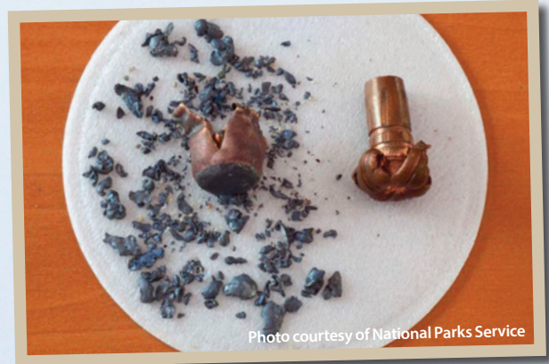
A recovered .270 caliber copper jacket lead-core bullet (left) is heavily fragmented compared to the solid copper bullet (right) that retained its original shape upon impact.
